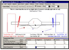
natural frequencies. Rear suspensions which can be analyzed include double A Arm, McPhearson Strut, 3 link with panhard bar, 4 link (3 types with panhard bar, diagonal strut, or angled links like the early Chevelle or late model Mustang), Z links or Watts linkage (special case of 4 link), ladder bars, truck arms, and C3 Corvette. The Full Vehicle version now also handles push rod and pull rod springs. Both versions now let you print the vehicle layout drawings from the main screen.
