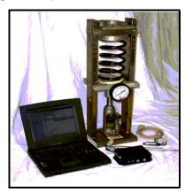
the Black Box will accurately record spring compression, force and time during one test stroke. This system will provide huge gains in accuracy, repeatability and time savings over manual testers. Sophisticated analysis software will then report open force, seated force.
