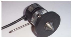
Ring magnet and rotary encoder ready to attach to end of camshaft.
