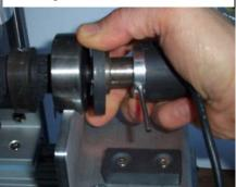
When done, the rotary encoder should be firmly attached to the camshaft, and the locating shaft held to the rectangular magnet. The cable should help hold the shaft securely on the magnet.
