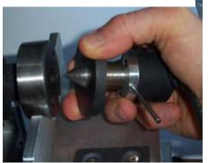
Insert the pointed Index into the end of the camshaft to firmly center the encoder, then release the magnet onto the camshaft.
