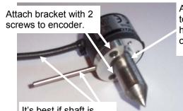
Attach pointed "index" to encoder with allen head screw on flat side of encoder shaft.
