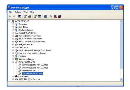
When the Device Manager window comes up, click on "Ports (COM & LPT1). Then you should see "USB Serial Port (COMX) were X is the Com Port number you should put in the COM Port number in the "Data Mite Specs"
